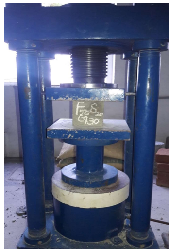
Fig 4.15 Compressive Strength Test
