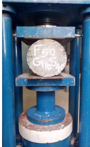
Fig 4.16 Split Tensile Strength Test
